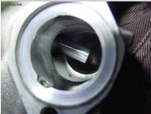
28 Now slide the actuator back out to install the timing piston. This is the final position of the actuator.
