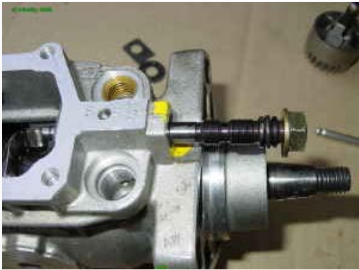
80 The governor adjustment screw.
