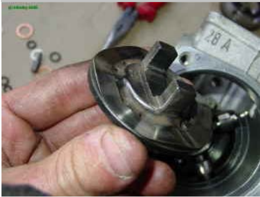
52 Put the cam disk in, completing the roller cage. Timing is adjusted by the slight rotation of the roller cage relative to the camplate.
