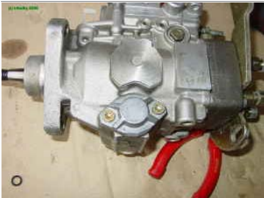
43 There are no controls for electrical coldstart on this car, so I put the usual cover on the cylinder.
