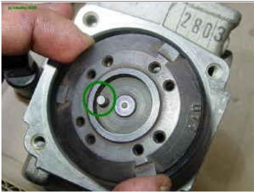
53 Note that the plunger drive pin (circled) aligns with the woodruff key of the driveshaft.
