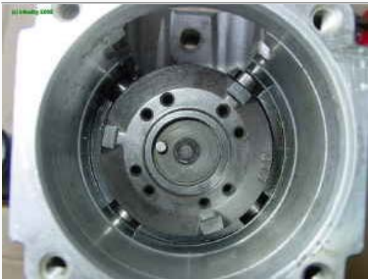
54 The cam lobes rolling on the cage cause the plunger to reciprocate and rotate simultaneously, building the high pressure for injection.
