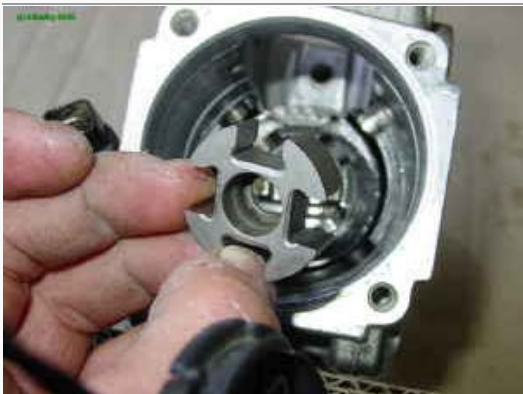
44 Insert the cross coupling that drives the rest of the pump.
