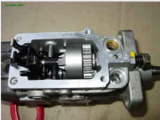
84 The adjustment of this shaft is important, because it modulates initial injection according to load (along with vacuum, if so equipped). This is why it is a good idea to mark its position at disassembly.
