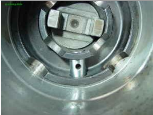
27 To understand how these systems interact, slide the timing pin into the crossover chamber so it protrudes into the timing cylinder. The pin controls the angular advance of the roller cage.
