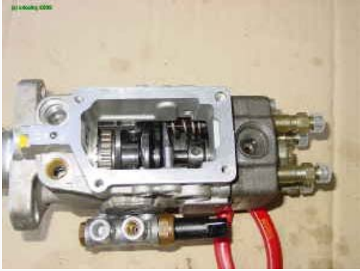
62 Insert the entire distributor head assembly into the pump, but don't tighten it down just yet.
